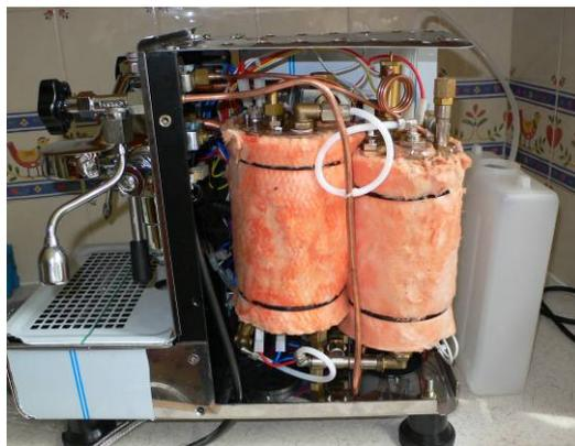
The twin boilers and water tank (removed)
