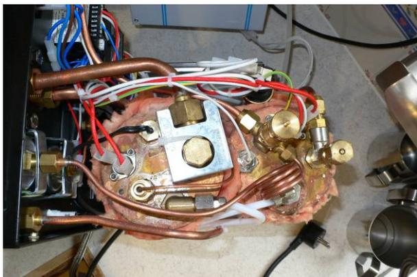
Top of the boilers with hi limit stats, vacuum breakers and safety valves
